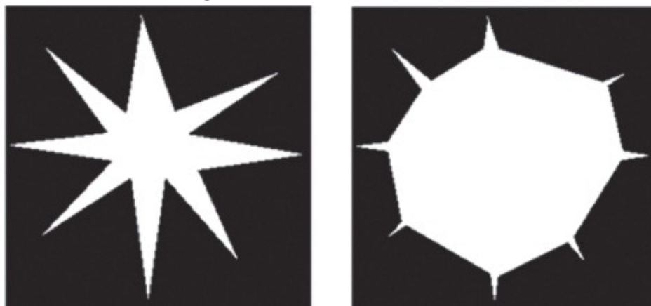
The hole on the right is bigger than that on the left, but the hole lining has got smaller
